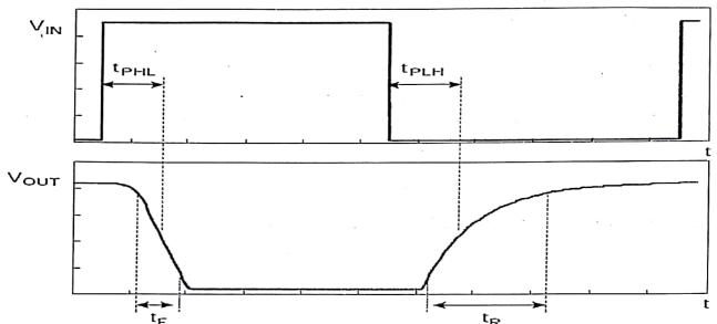
Transient response for an inverter with a rectangular input waveform.
