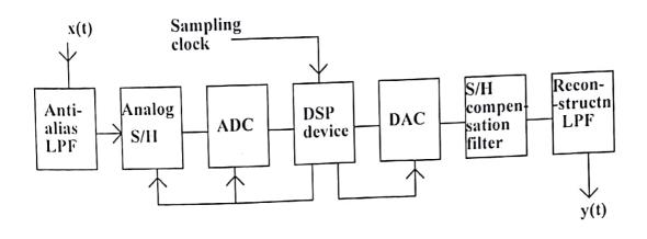
Antialiasing LPF: Analogue low-pass filter with cut-off frequency less than half the sampling frequency (fs) to remove (strictly, to sufficiently attenuate) any spectral energy of the input signal x(t) above fs/2. When x(t) is sampled, this spectral energy would otherwise produce, by aliasing, lower frequency energy capable of distorting the digitised input signal in the frequency range 0 to fs/2.
