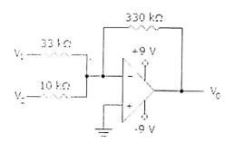
$$V_0 = -R_f \left( \frac{VI}{R_1} + \frac{V_2}{R_2} \right)$$
