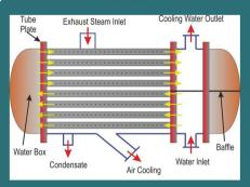
condenser is а aadaet, substances are where vaporous compressed into a fluid state cooling utilizina a aaent then, at that point, latent heat is released in the climate, also It lessens the back pressure of the steam, and subsequently, more work can be acquired, and may it's types include HVAC air curls.
