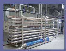
suitable for heating or cooling small flow rates of fluids. They are cheap, have a flexible design, and are easy to maintain. They can be constructed from pipes of the same lengths interconnected with fittings at the ends to maximize floor space, it structure is simple, and the heat transfer area can be increased or decreased freely.
