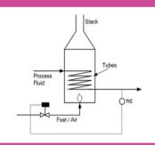
Heater is used to transfer heat a heat source to medium or that needs to be heated. there are different types of heaters. they differ their design, mode of operation and applications. Electric water heaters. Gas heaters. Steam heaters. and Thermal oil heaters.
