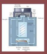
Is device which heat and vaporize a working fluid. In many cases, they are similar to industrial boiler except that they do not build up high pressures. Vaporizer units are most commonly used for low pressure heat transfer by incorporating the vaporized stream as the heat exchange fluid. also used to vaporize liquid fuels or cryogenic liquids.
