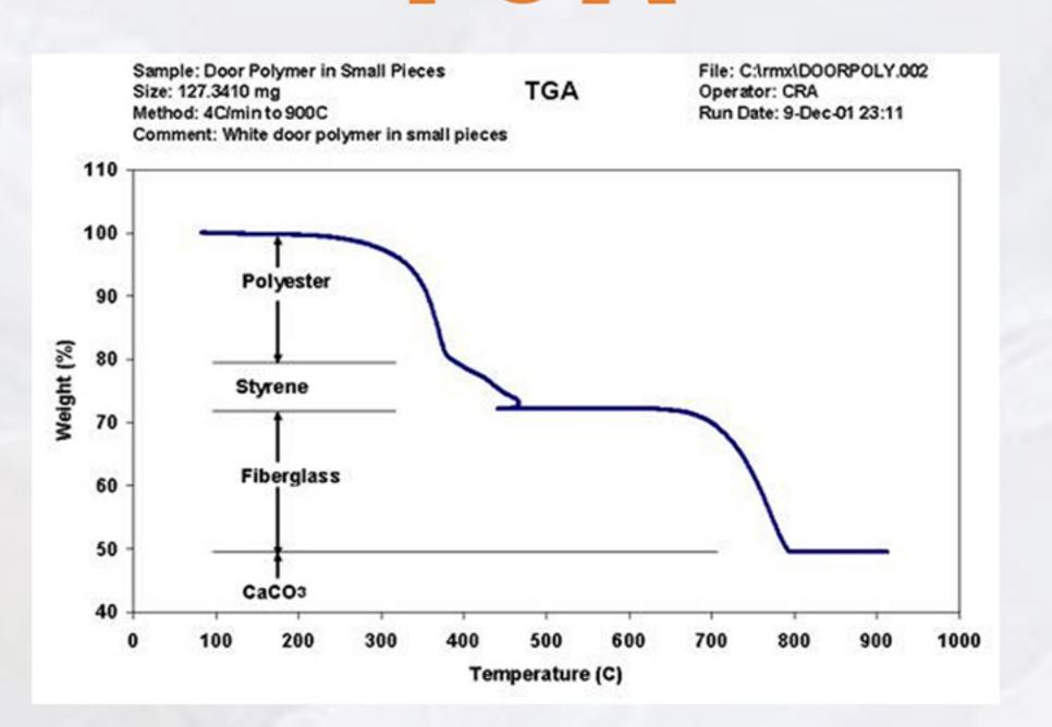
Thermogravimetric analysis (TGA) measures weight changes in a material as a function of temperature (or time) under a controlled atmosphere. Its principle uses include measurement of a material's thermal stability, filler content in polymers, moisture and solvent content, and the percent composition of components in a compound.
