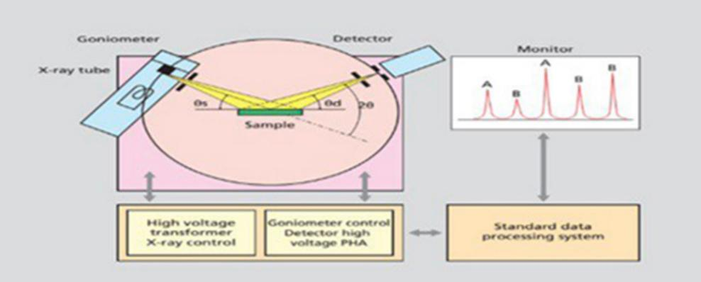
The XRD (X-ray Diffraction) device is used to study the structure of crystals and determine their atomic arrangements. The operation of the XRD device is based on the principle of X-rays interacting with the crystalline lattice structure of materials.
