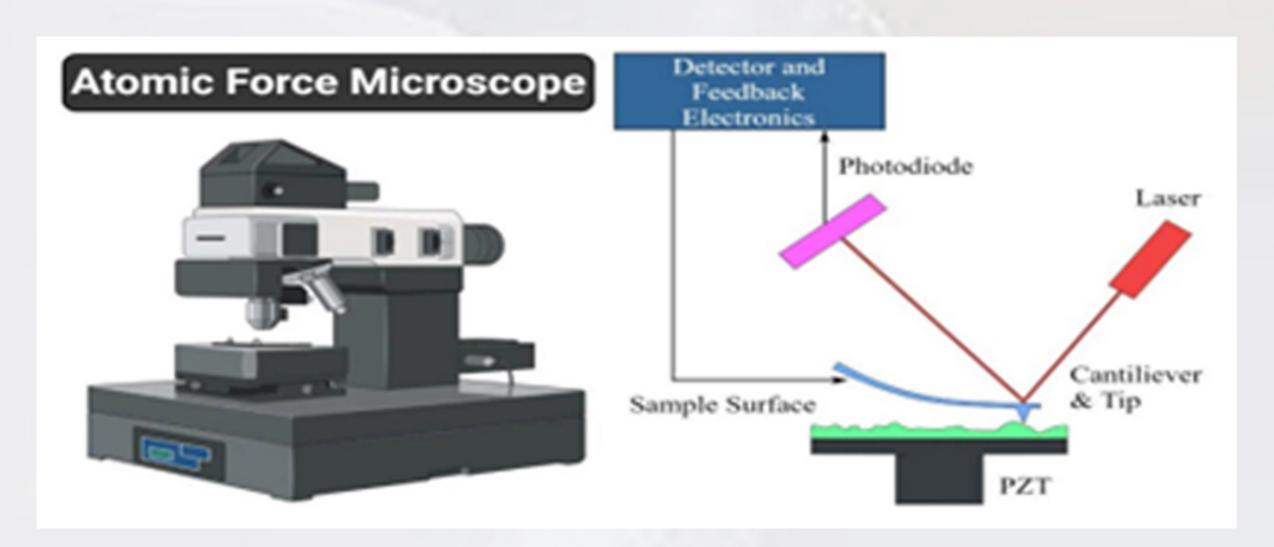
The Atomic Force Microscope (AFM) is a device used in nanotechnology, biology, and physics to visualize objects at the atomic and molecular level. This device creates high-resolution three-dimensional images of objects on their surfaces.
